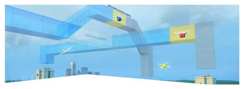
▲ This image depicts one scenario FAA plans to test during flight tests under the UAS Traffic Management program to create a traffic management scheme for drones flying below altitudes of 400 feet, which current air traffic services do not cover. Among the scenarios explored during flight tests was rerouting drones to avoid collisions with other aircraft.
