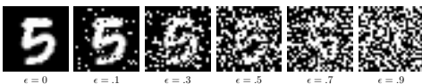
Fig. 5. A template image shown with varying noise densities \epsilon which represents the fraction of pixels that are impacted by noise.
